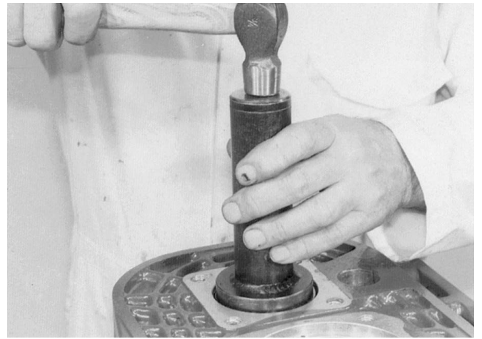
23. Drive out the outer cup from the layshaft rear bearing. Use tool N° 007.
