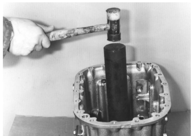
25. Drive out the front bearing from the main shaft. Use a tube.
