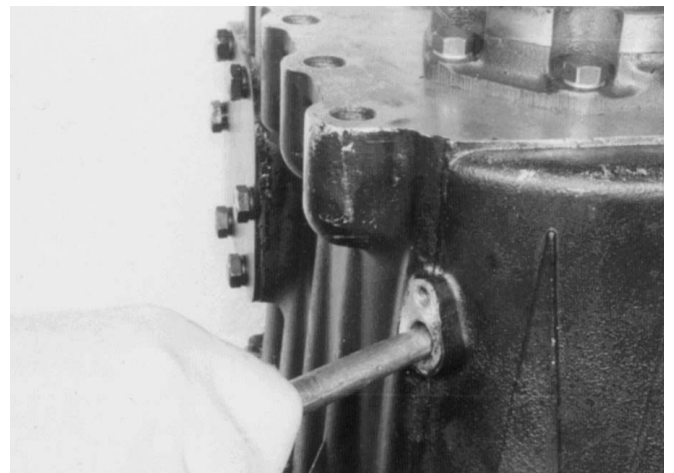
16. On overdrive models, using a suitable probe (as illustrated), align the pivot pins with the holes in the casing. Apply sealant (Loctite 518) to the pivot pin flanges and insert the pins.
