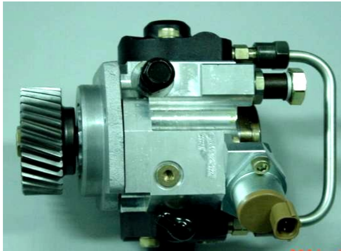
Fuel supply pump
