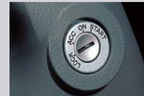
Double Locking System The basic feature deters theft and prevents accidental starting.
