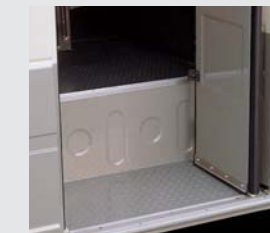
Door Step Step surfaces is textured to prevent slipping when wet.
